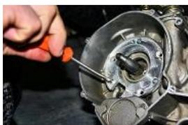
**PRESENTER LA PLATINE PREMIUM ET LA SERRER AVEC 3 VIS FOURNIES AVEC UN TOURNEVIS CRUCIFORME**
