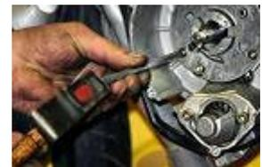
**ATTENTION ! LES 3 VIS DE LA PLATINE SONT PARTICULIEREMENT DIFFICILES A DESSERRE ! POUR SE FAIRE PRESENTER UNE CLE ALLEN DE 3 ET TAPOTER AVEC UN MARTEAU SUR LA CLE**
